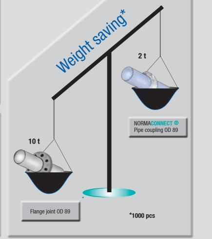
The NORMACONNECT® FGR range offers reliable weld-free connections for thickand thin-walled pipes and conforms to the new standard DIN 86128.
